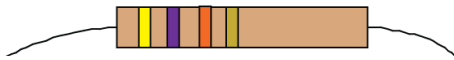
FIG. 4: The upper panel shows the resistor color codes. The first digit of the resistance in the lower panel is a 4, the second digit is a 7 and the multiplier is a 3, so the resistance is R = 47 \times 10^3 \Omega . The fourth color is used to calculate the uncertainty in the resistance. The tolerance of this resistor is 5% (corresponding to the gold band). The uncertainty in the resistance is given by: uncertainty = R \times \text{tolerance} = 4.7 \times 10^4 \Omega \times 5/100 = 2.35 \times 10^3 \Omega .
