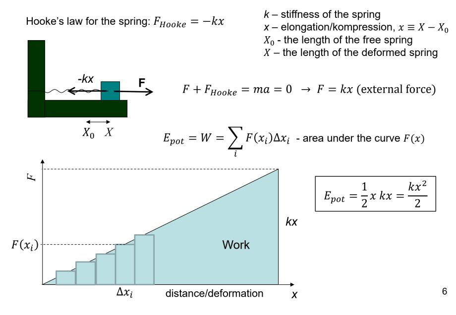
In the absence of dissipation (friction) the total energy of an isolated system is conserved:
