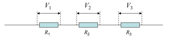
As the current I through each of serially connected resistors is the same, one can use Ohm's law and write
