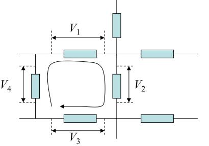
$$V_1 + V_2 + V_3 + V_4 = 0$$
