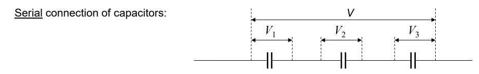
Here voltages add up whereas the charge is common (on each of the capacitors the same)
