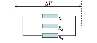
Here the potential difference V is common for all resistors, whereas total current is the sum of individual currents:
