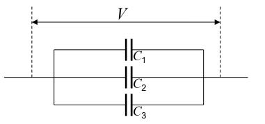
Several capacitors connected in parallel form an effective capacitor *C* whose charge is the sum of the charges on all capacitors, whereas the voltage is common:
