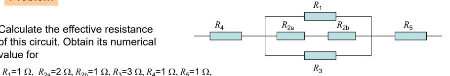
Solution: We at first replace the serially connected resistances  $R_{2a}$  and  $R_{2b}$  by the effective resistance  $R_2 = R_{2a} + R_{2b}$ . Then we replace the central group of parallel connected resistances by the effective resistance <u>∖</u> −1
