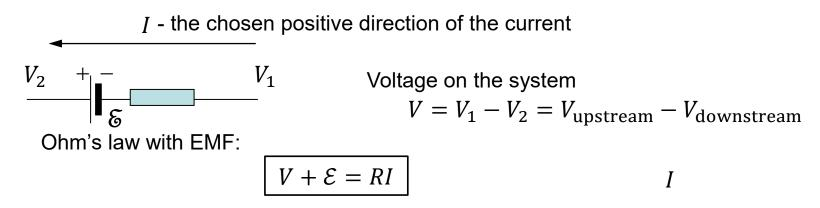
Consider the simplest closed circuit: battery and the load.
