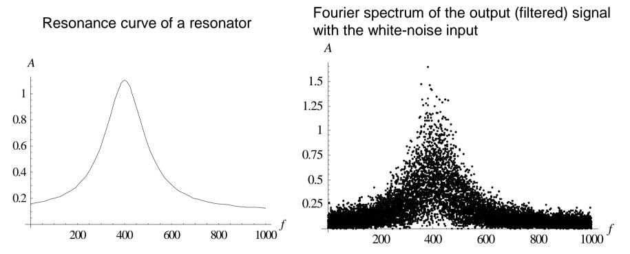
The output signal is not the <u>white noise</u> but a <u>colored noise</u>. It has a maximum at the resonance frequency (here  $f_0=400$  Hz), so that the ear can hear this frequency above the hiss.
