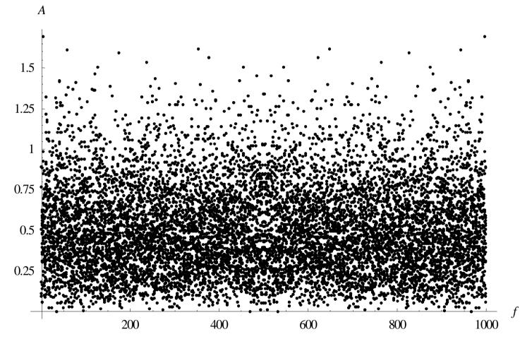
Note: In wave editors like Audacity, the Fourier spectra of sounds are <u>smoothed</u> (that is, averaged over some small frequency range around any particular frequency) for a nicer presentation. As a result, the Fourier spectrum of the noise looks like the idealized Fourier <sup>5</sup> spectrum above.
