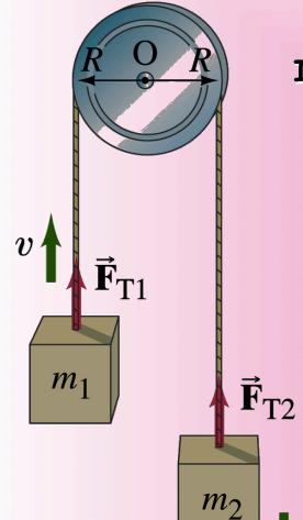
If the system is now released, use conservation of energy to determine the speed of m<sub>2</sub> just before it strikes the ground.
