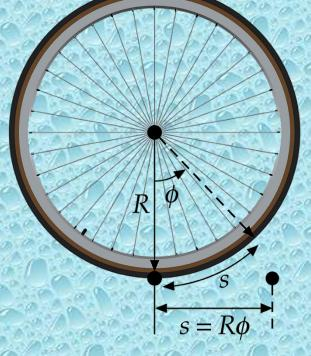
A wheel of radius R is rolling without slipping along a straight path. As the wheel rotates through an angle Ø the point of contact between the wheel and the surface moves a distance s that is related to Ø by
