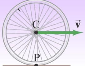
The same wheel is seen from a reference frame where C is at rest Now point P is moving with velocity -v The linear speed of the wheel is related to its angular speed
