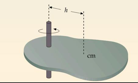
Let I be the moment of inertia and let  $I_{cm}$  be the moment of inertia about a parallel-axis through the center of mass. Let M be the total mass of the object and h the distance between the two axes. The parallel axis theorem states that
