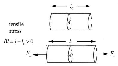
Figure 26.2: Tensile stress on a rod
