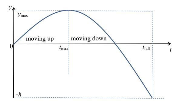
b) The time dependences of the velocity and displacement in the motion with constant acceleration are given by the formulas
