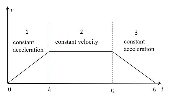
Segment 1. Time from 0 to  $t_1$  (unknown), acceleration  $a_1$  = 3 m/s<sup>2</sup>, final velocity  $v_1$  = 15 m/s.
