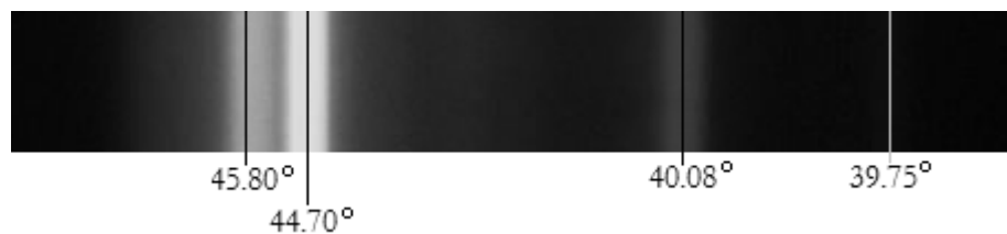
Figure 19.2 A typical diffraction pattern for one fringe from the light emitted by Mercury
