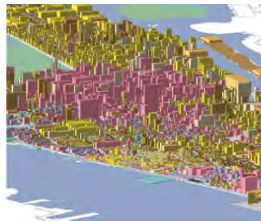
Figure 12.3b A lot-level 3-D image of midtown Manhattan, using building heights (from an attribute database) as the third dimension.
