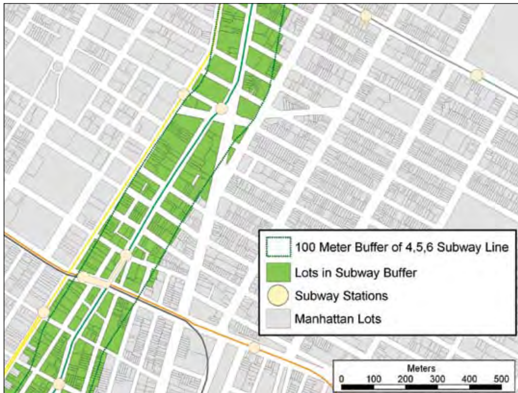
Figure 8.3 The results of a spatial query: a buffer shows properties that lie within 100 meters of a subway line.
