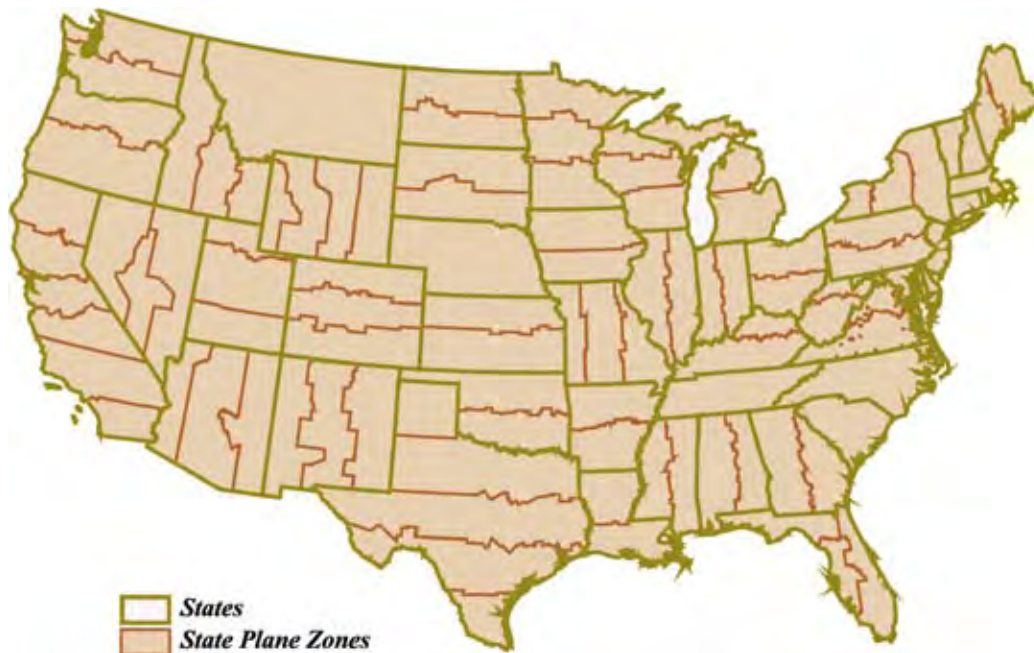
Figure 2.19 State plane zones of the fifty states show how their orientation depends on whether the state is east–west trending or north–south.
