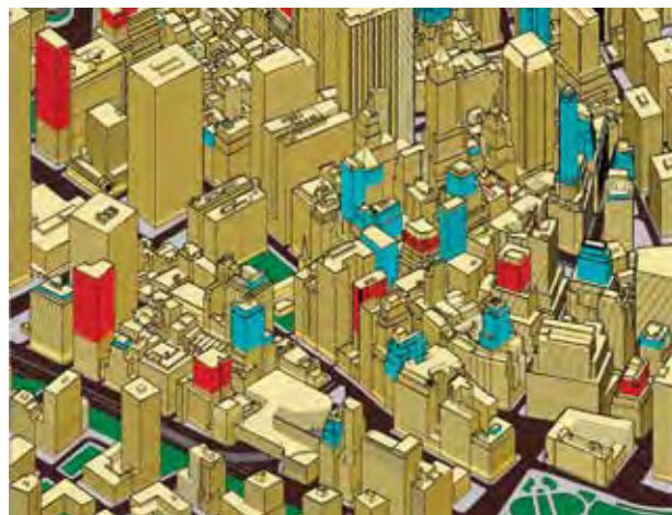
Figure 12.3a A three-dimensional GIS model of buildings in downtown New York, with attribute data displayed thematically by color. Colors show floors above the fourteenth floor, with a square footage of 8,000 or less. Red indicates floors in buildings that are 8,000 square feet or less; cyan indicates floors in buildings completed prior to 1945.
