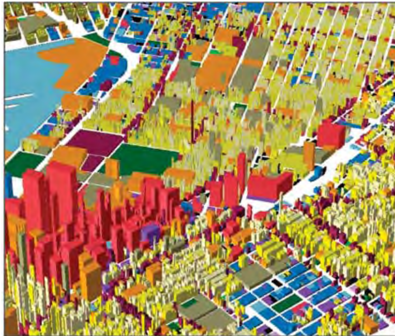
Figure 12.4 Using the third dimension to represent the non-spatial attributes of geographic entities: assessed total value of lots in downtown Brooklyn, color-coded by land use.
