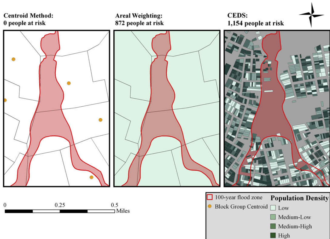
Fig. 9. 100-Year flood zone in a small area of Staten Island, NY showing population densities calculated with the centroid-containment method (left), areal weighting (center) and CEDS (right). The centroid-containment method predicts zero people since no centroids fall within the flood zone. AW not only predicts fewer people than CEDS, but also different people.
